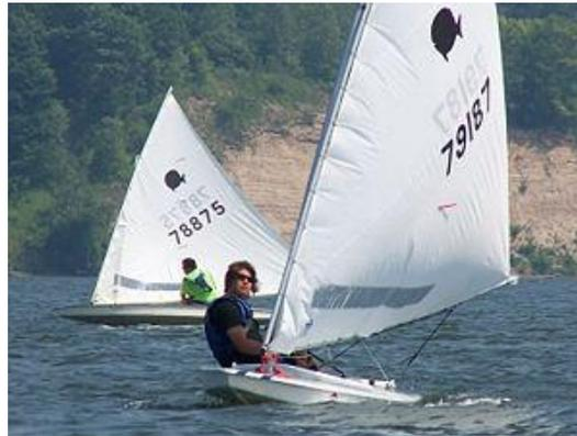
A race rigged Sunfish racing on Irondequoit Bay, NY. The rig is carried lower to the deck and additional lines are added to control sail shape
