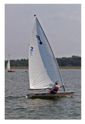
The Force 5 is a powerful single-handed racing dinghy. Although one person races the boat, the cockpit is large enough to accommodate two people and provide ample day sailing enjoyment. This 14' craft has a 91 square-foot mainsail, rolled deck and an adjustable rig. It is easily car topped. The class association website is www.force5.us.
