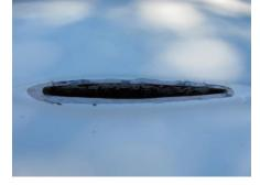
all the way into the slot and is perfectly centered in the boat. Secure that centering with a line to each side so that it won't move while working. Work fast, as body putty dries quickly. When dry, remove board and make sure that it slides up and down easily. Sand the inside of the slot if needed. Then at the upper end of the slot, I'm currently using foam padding after trying a rubber gasket for a few years. You can also glue in some carpeting to keep the board from wobbling side to side.
