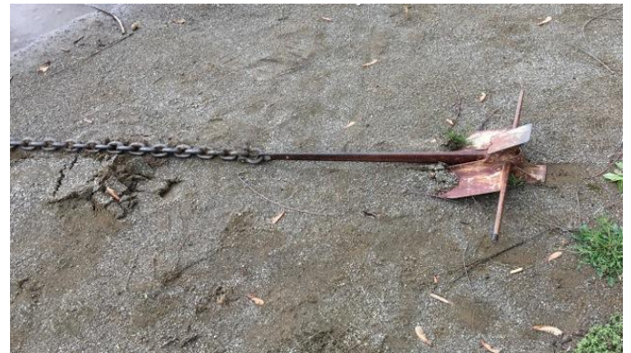
(Fig 2) Five feet of heavy anchor chain helps keep the anchor flat on the bottom of the lake so the pointed flukes can dig into the mud to hold the boat.
