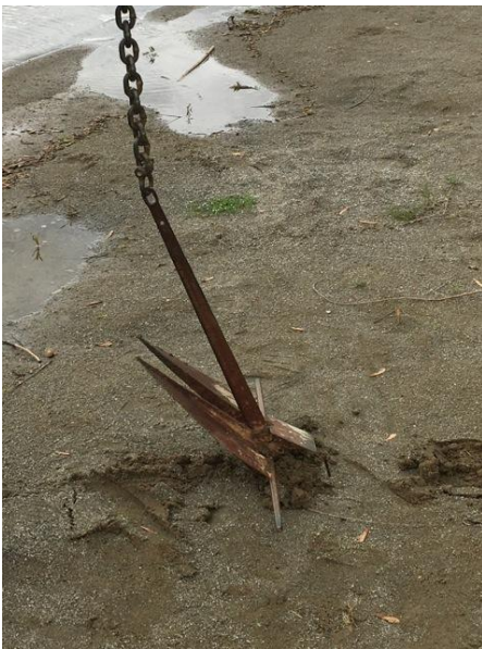
(Fig 2) Five feet of heavy anchor chain helps keep the anchor flat on the bottom of the lake so the pointed flukes can dig into the mud to hold the boat.
