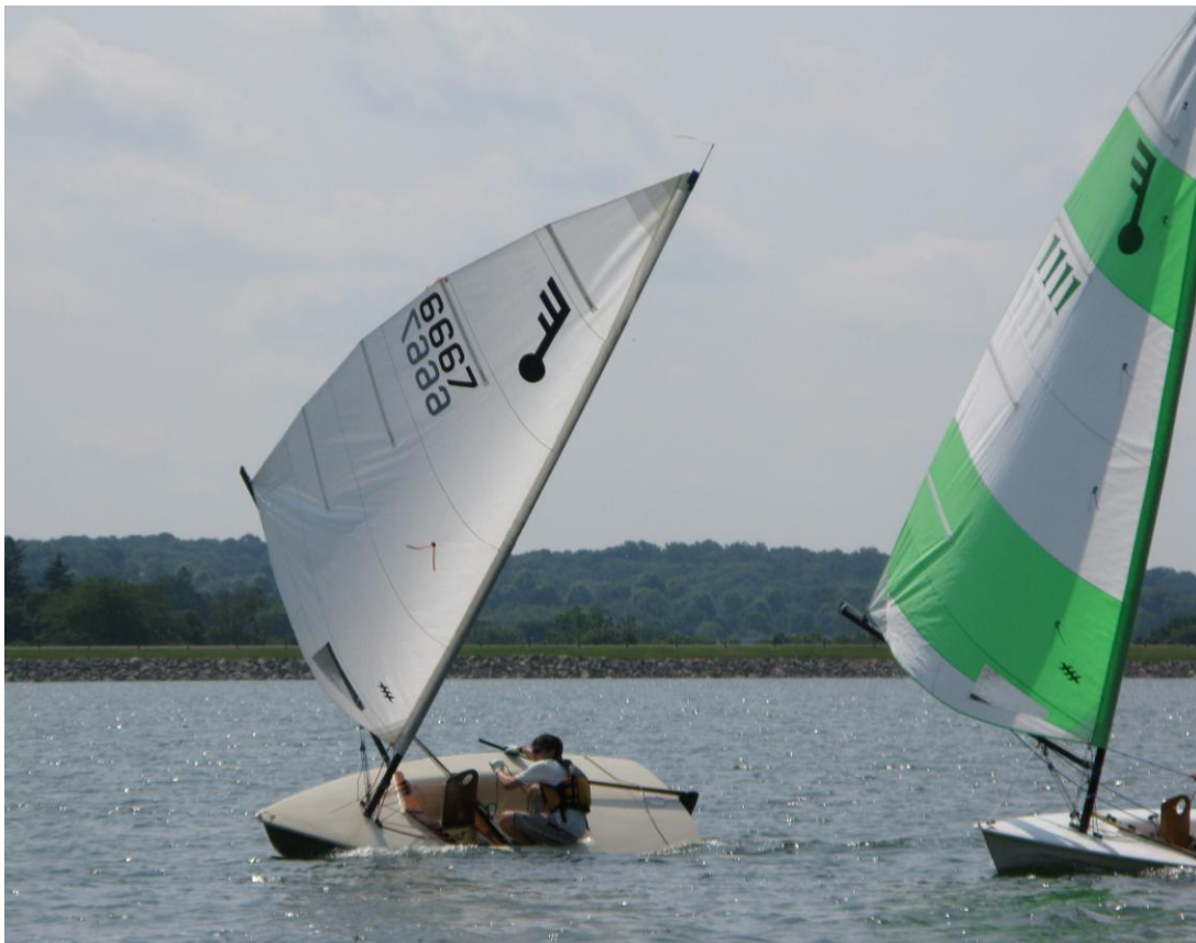
Heeling to windward while sailing downwind reduces weather helm and wetted surface. HSC's Caleb Zimmerman (6667) is shown testing the limits of the technique. Photo by Anne Freeman
